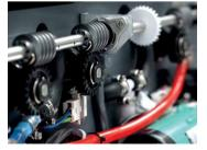
InterPlater MD uses a worm drive system, well known from the InterPlater HDX, for driving rollers and brushes.
