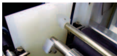
Gum applicator The gum applicator roller can be flipped up during shut-down periods to avoid sticking together.
