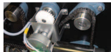
Bristle brush motor Individual motor for bristle brush in wash section.
