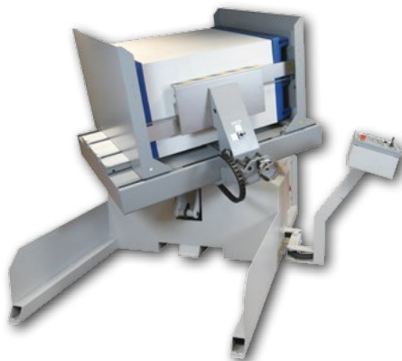
3. Turning pile in airing position
